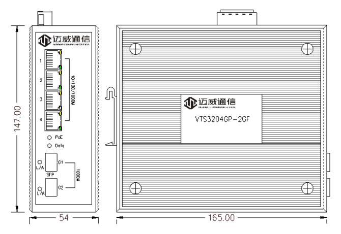
Din-rail mounting (Unit: mm)
