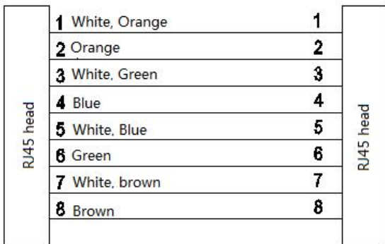
CAT. 5 straight line cable connection method
